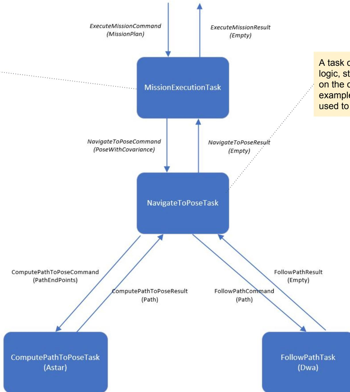
A task can coordinate subtasks using hand-coded logic, state machines, or behavior trees, depending on the complexity of the task coordination. For example, a simple BT sequential node could be used to sequence tasks:
